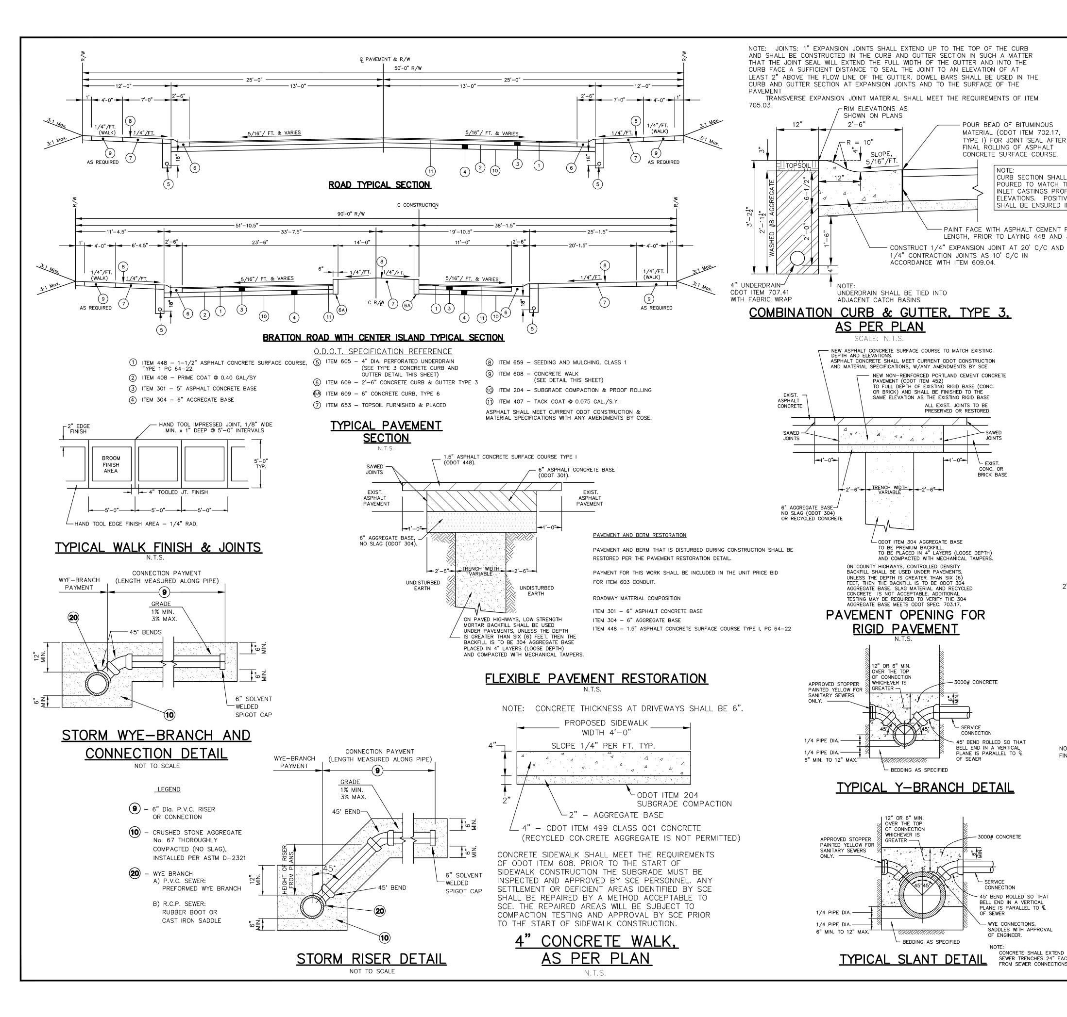
NOTE: JOINTS: 1" EXPANSION JOINTS SHALL EXTEND UP TO THE TOP OF THE CURB AND SHALL BE CONSTRUCTED IN THE CURB SECTION IN SUCH A MATTER THAT THE JOINT SEAL WILL EXTEND THE FULL WIDTH OF THE GUTTER AND INTO THE CURB FACE A SUFFICIENT DISTANCE TO SEAL THE JOINT TO AN ELEVATION OF AT LEAST 2" ABOVE THE FLOW LINE OF THE GUTTER. DOWEL BARS SHALL BE USED IN THE CURB AND GUTTER SECTION AT EXPANSION JOINTS AND TO THE SURFACE OF THE PAVEMENT
