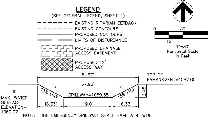
NOTE: THE EMERGENCY SPILLWAY SHALL HAVE A 4' WIDE CONCRETE SECTION EQUAL TO THE 4" CONCRETE WALK ON DETAIL SHEET 74, WITH A MEDIUM BROOM FINISH CENTERED IN THE SPILLWAY ACROSS THE LENGTH BETWEEN MAXIMUM WATER SURFACE ELEVATIONS.
