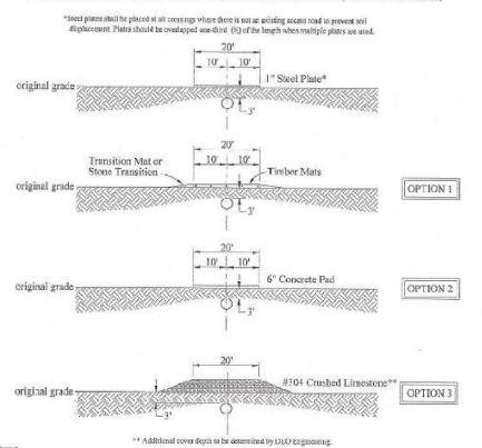
1) Agency/person requesting to cross must submit detailed load information 2) All mitigation options (1, 2 and 3) require DEO Engineering approval. 3) Low ground pressure equipment such as trackhoes and buildozers may not require mitigation. ) Impact loads can be caused by dropped objects and should be avoided. Crossing speed should be as low as possible.
